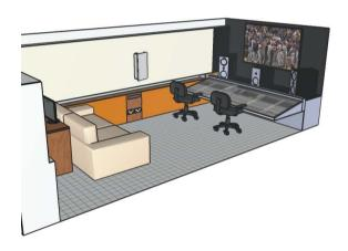
The truck can be used for live to cinema transmissions as well at traditional broadcast activities, both of which require a different monitoring setup. We have installed a recallable monitoring system to facilitate optimum results in either situation. Using FIR filters, each speaker can be eq'd and the level changed with no discernible loss of audio quality. The preset can be saved to a USB stick for subsequent use.
